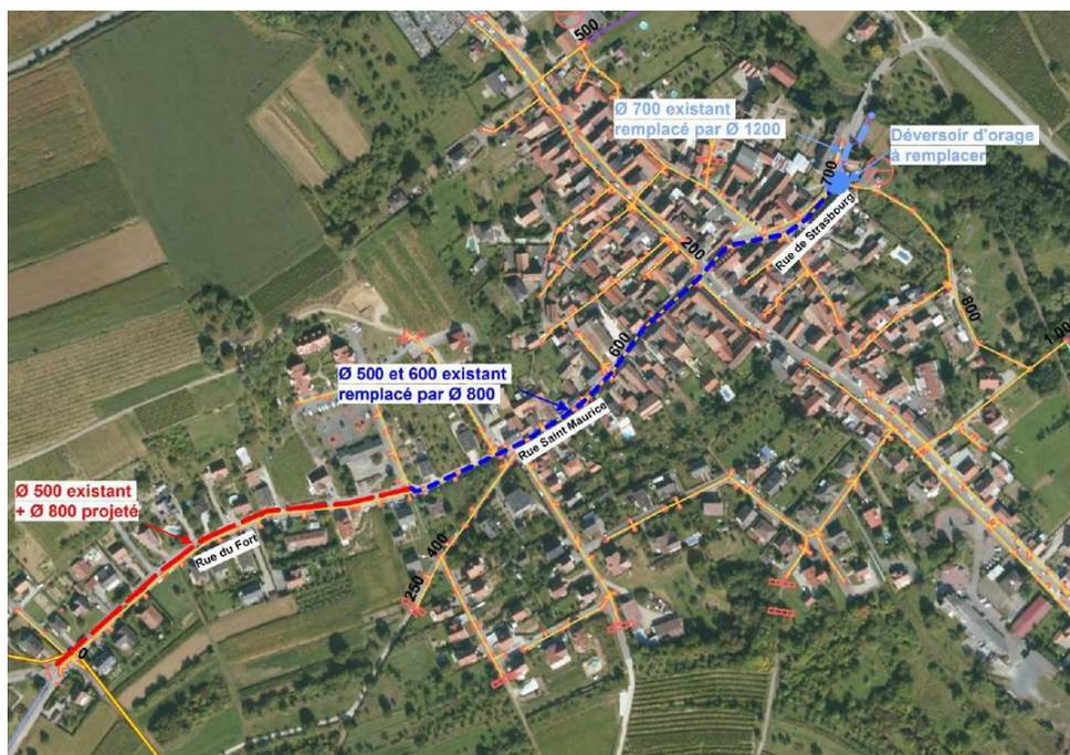
Fig. 23. PROPOSITION DE RENFORCEMENT DU RESEAU D'ASSAINISSEMENT
